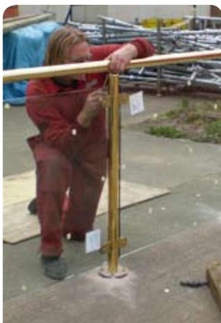
Balustrade components were assembled for testing. These included:
