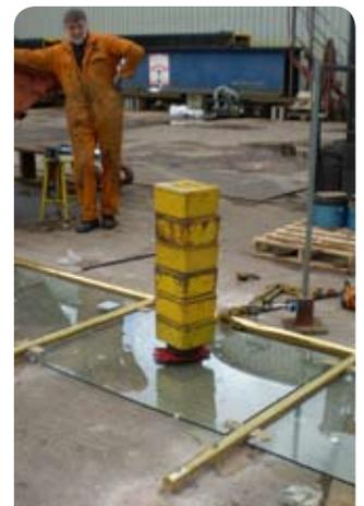
Image shows testing for 'Point load applied to infill'.
