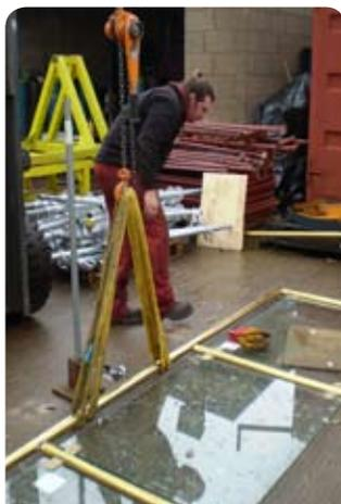
Systems were tested for 'Horizontally uniformly distributed line load'.
