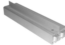
Service position double top rail to be fitted between two-service position posts (with baffles fitted). Rebate has a 30mm space each of the rail to allow for the sound baffles.
