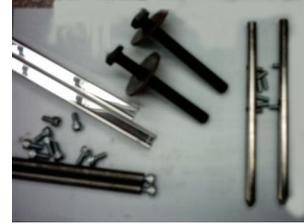
Vertical post sections of the framework. The posts are supplied as ends, centres or corners as required. Service position posts are supplied with fitted sound baffles.
